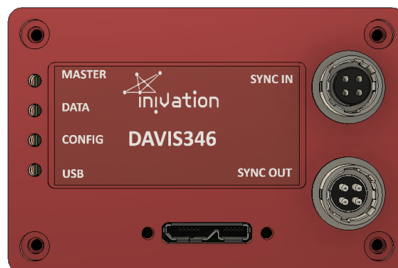
Figure 2 Connectors on the back of DAVIS 346
