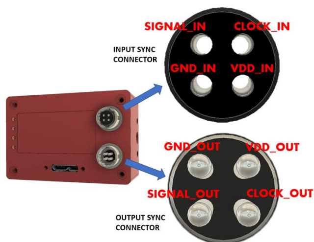
Figure 3 Sync connector pinouts on DAVIS 346
